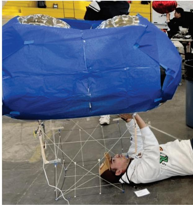
**Figure 10.** Photo of IU Autonomous Sports class prototype LTA vehicle while a student replaces the battery.
