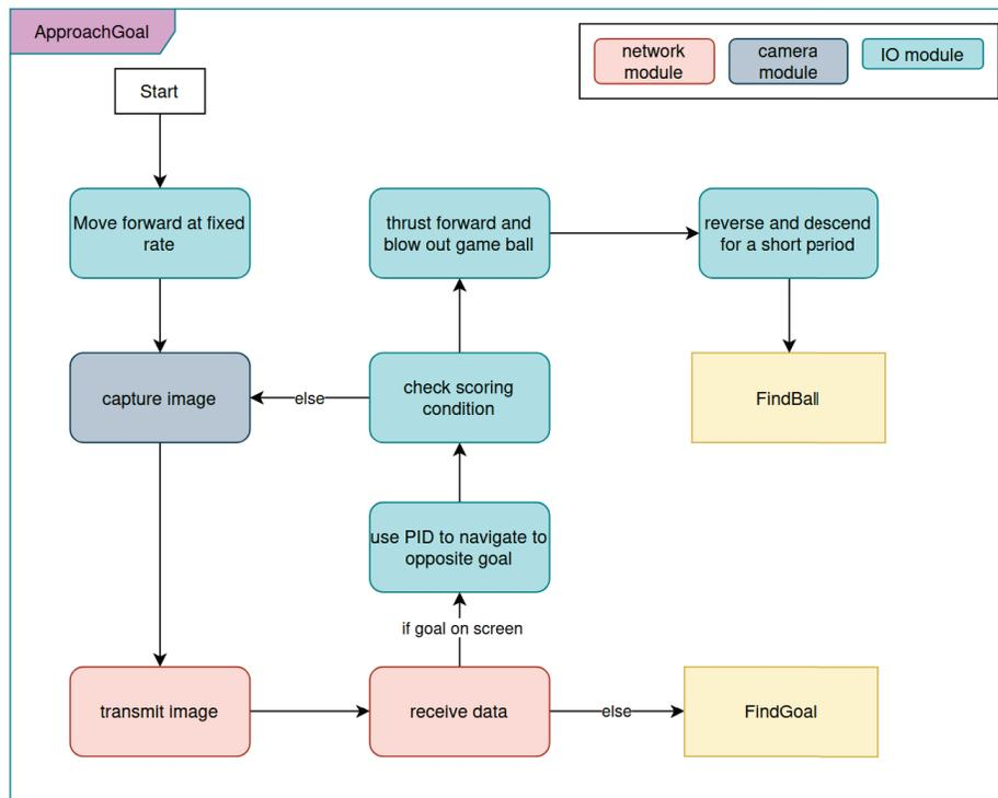
Figure 16. Flowchart for the actions and conditions during the "approachGoal" state in the state machine.
