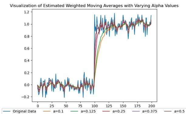
Figure 15. Graph displaying various levels of EWMA filtering for a noisy step function.
