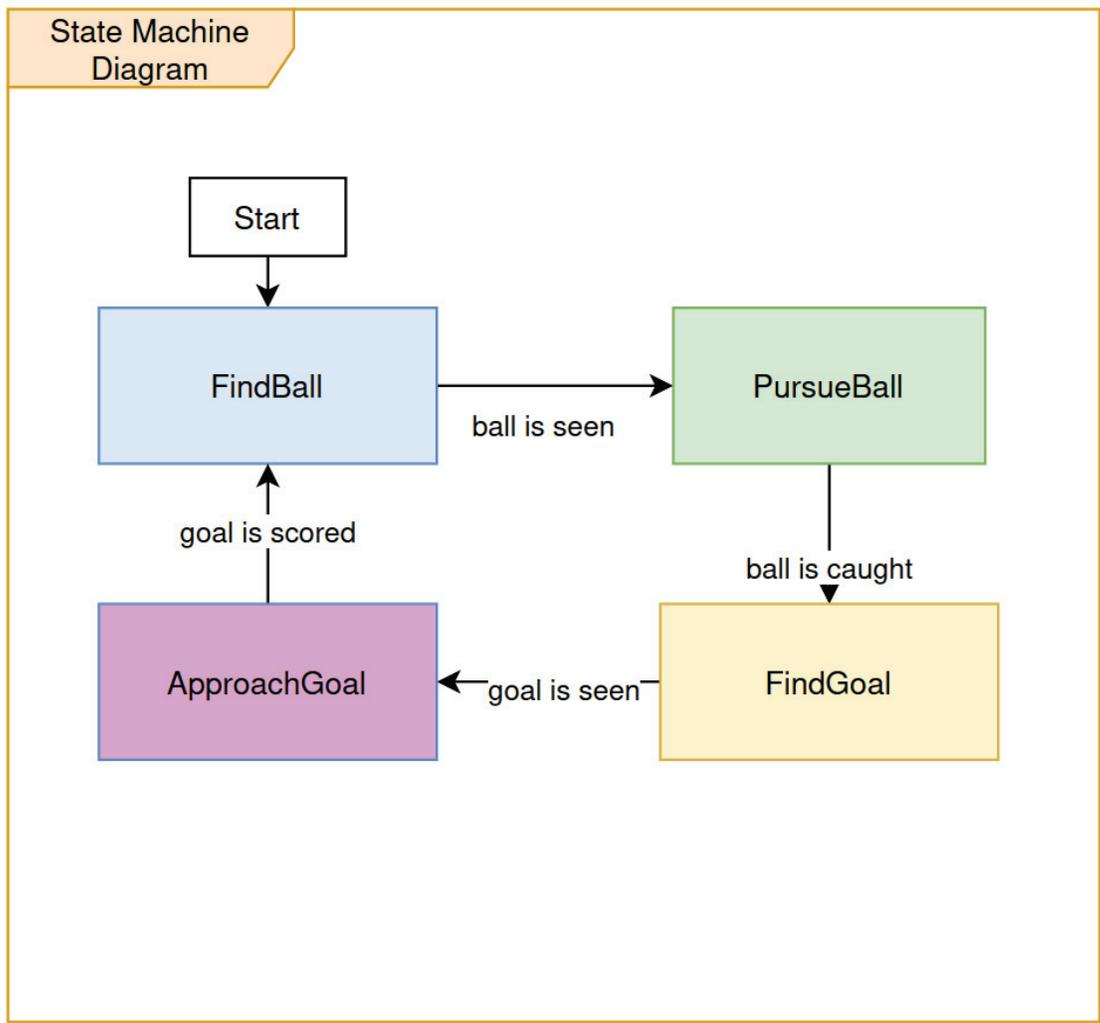
Figure 13. A flow chart diagram of the discrete state machine for the blimp.
