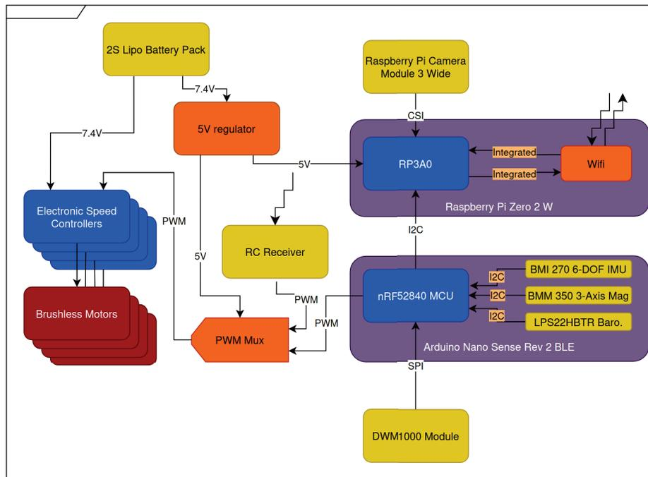
Figure 12. Hardware system diagram for the design of Indiana University's blimp.
