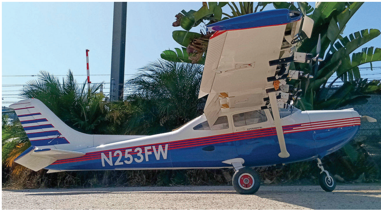
Figure 6. Modified 35% C-182 Subscale Research Aircraft.
