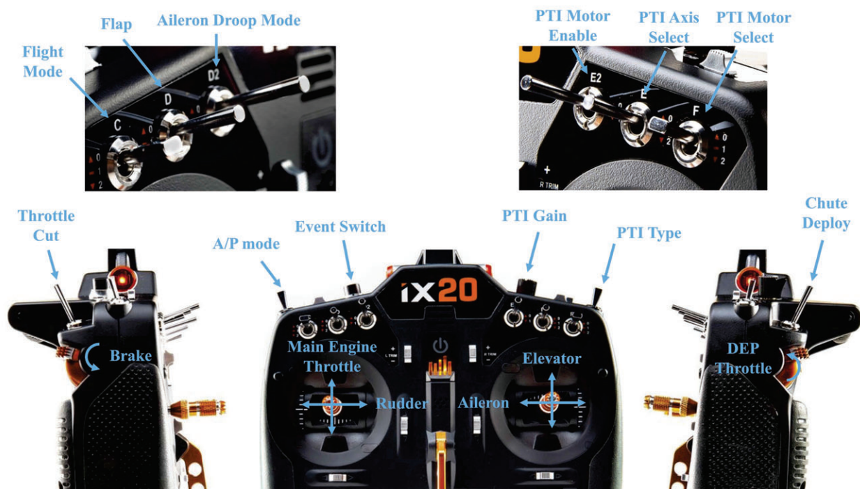
Figure 29. Layout of transmitter controls.
