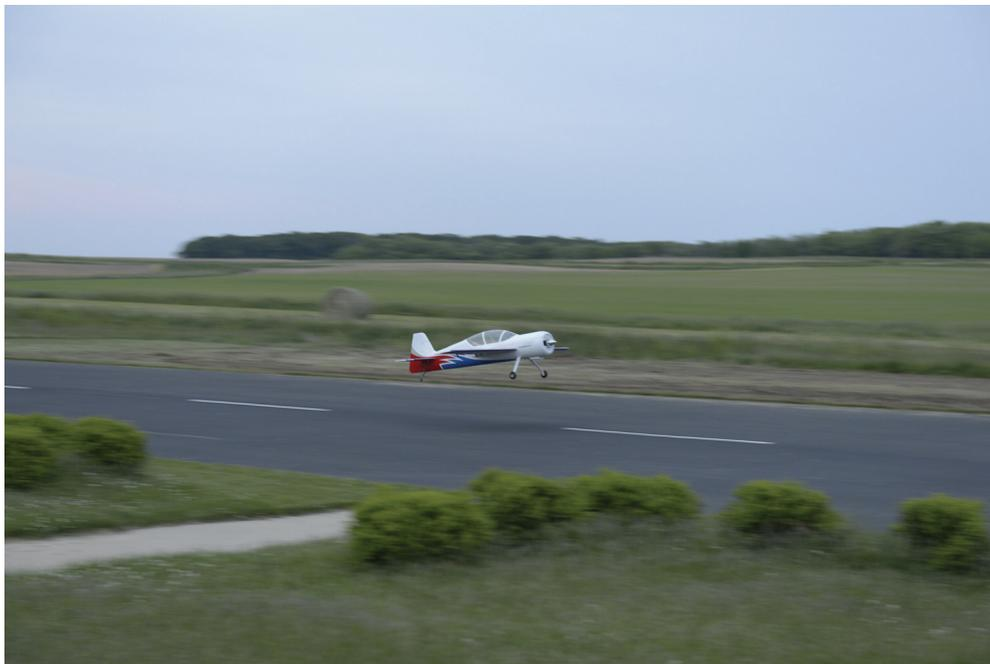
Figure 14. The UIUC Subscale Sukhoi aircraft landing.
