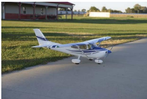
Figure 1. The baseline GA-USTAR aircraft (1/5-Scale Top-Flite Cessna 182).
