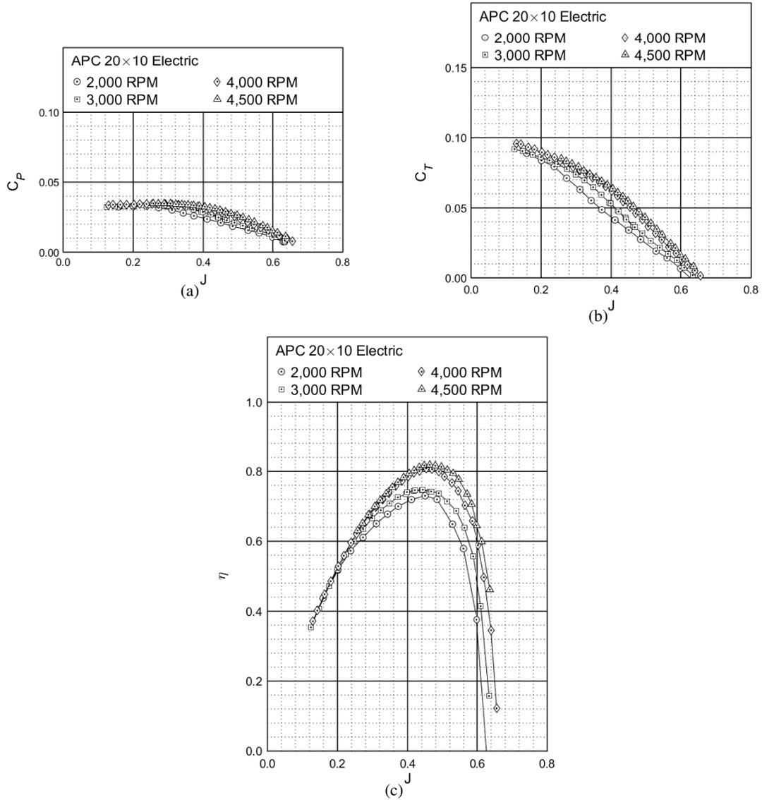
Figure 10: Performance of the APC 20×10 Thin Electric propeller: (a) thrust coefficient, (b) power coefficient, (c) efficiency.
