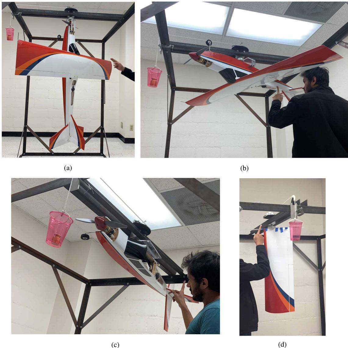
Figure 7: Moment of inertia measurement of the flight-ready, instrumented Avistar UAV about the (a) roll axis, (b) yaw axis, and (c-d) pitch axis.
