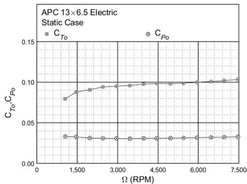
Figure 9: Static performance of the APC 13×6.5 Thin Electric propeller: thrust and power coefficient.
