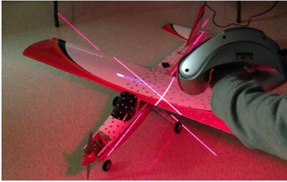
Figure 5: The Avistar UAV being 3D scanned from above.
