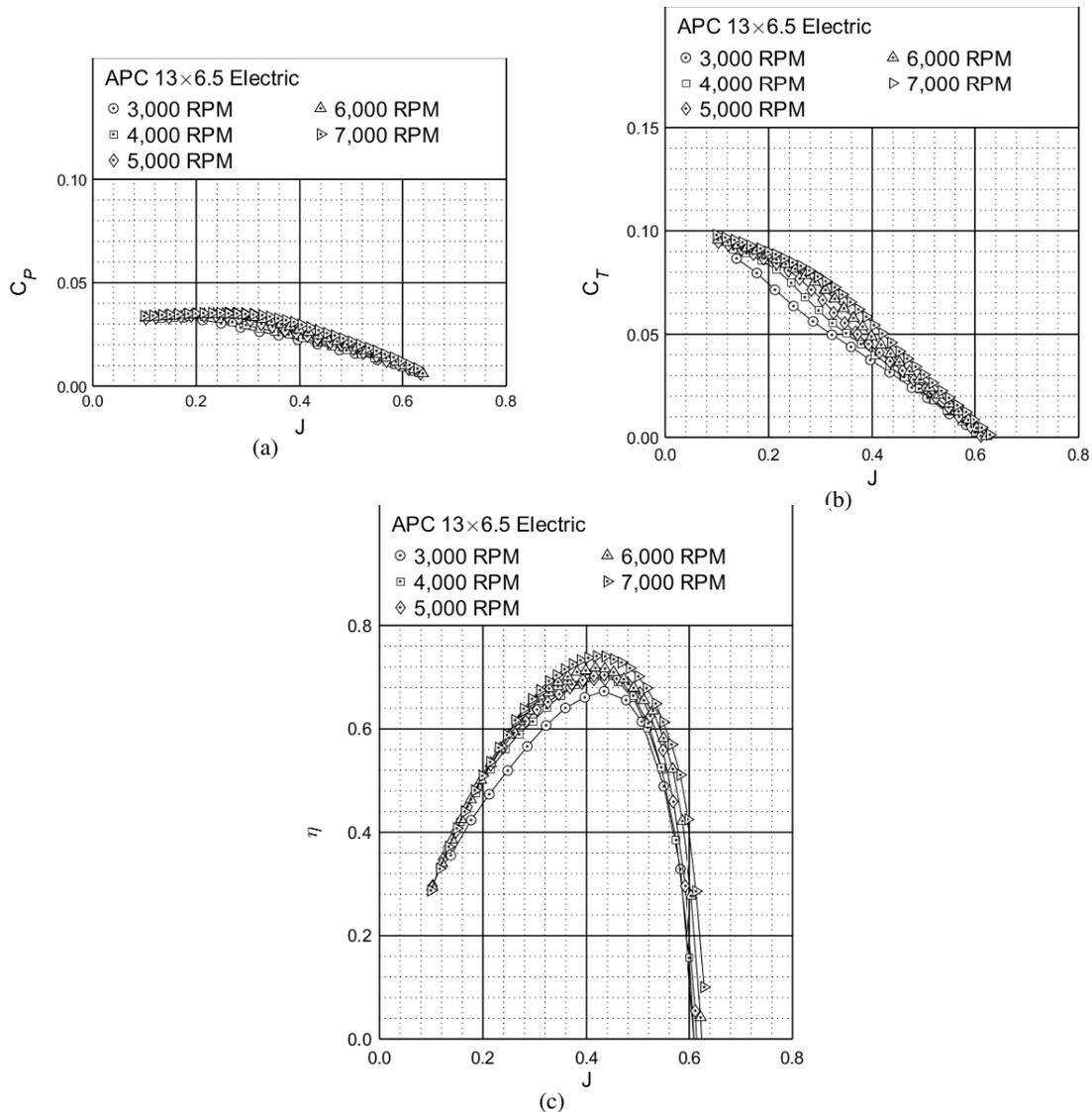
Figure 8: Performance of the APC 13×6.5 Thin Electric propeller: (a) thrust coefficient, (b) power coefficient, (c) efficiency.
