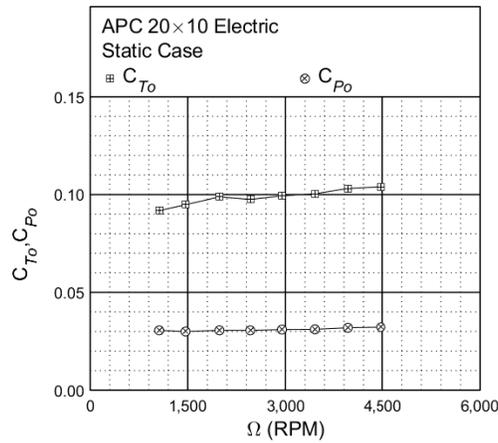
Figure 11: Static performance of the APC 20×10 Thin Electric propeller: thrust and power coefficient.
